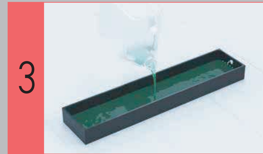
3 Pour the diluted solution into the trough. Do not overfill!
